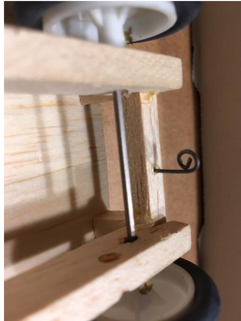
Figure 5. Wire curved with pliers and inserted into wood
